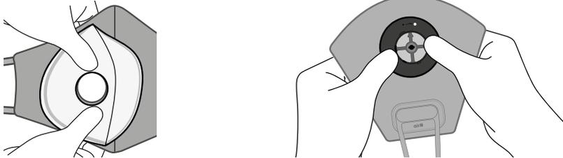
Align both the inner filter and the outer mask by the hole. Assemble the air valve at the hole.
