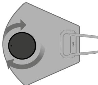
Align the dots on Bracket ② and Air Valve Cover in a linear position.
