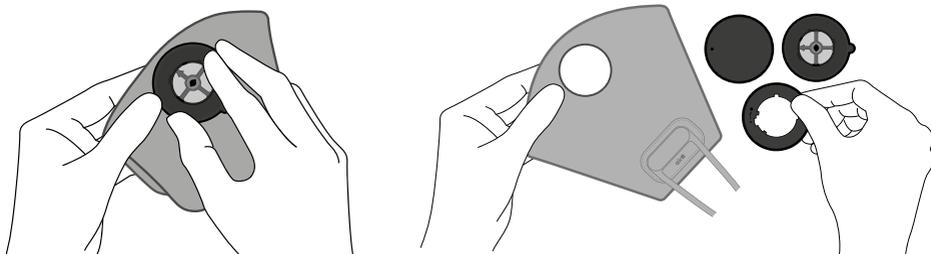
Detach the bracket from the mask to remove all remaining air valve components.
