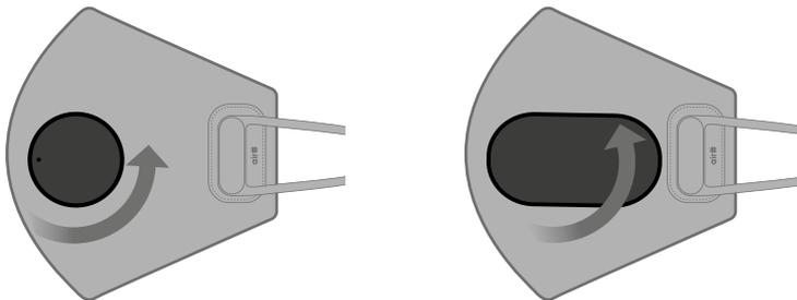
To remove the air valve or the fan unit\*, detach by rotating counterclockwise.
